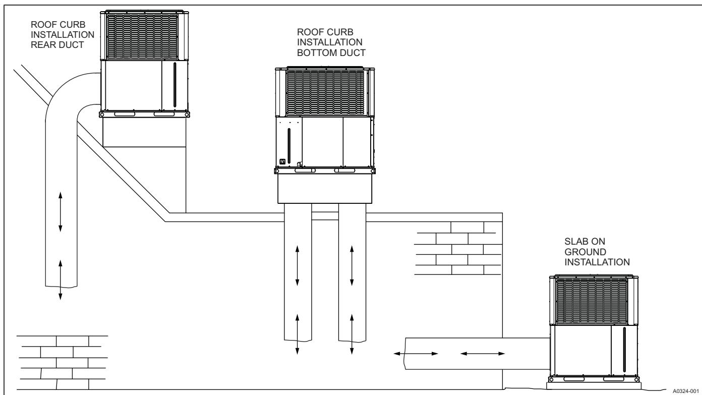
**UNIT TYPICAL SLAB ON GROUND INSTALLATION**
