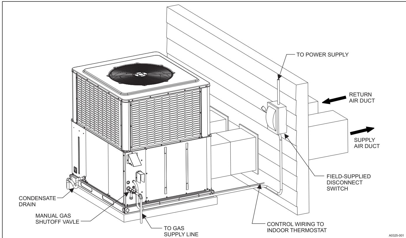
**UNIT TYPICAL ROOF CURB INSTALLATION**
